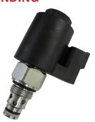
2/2 Pilot operated poppet type Normally closed Max. pressure: 350 bar (5000 psi) Max. flow: 40 lpm (11 gpm)
