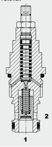
The DB12P is a pilot-operated, spool type pressure relief valve. If the pressure at port 1 exceeds the pressure setting, the pilot poppet opens, creating a small flow over the orifice of the pilot stage to the tank. The pressure drop across the orifice lifts the main spool against a light spring, opening the connection between port 1 and port 2.
