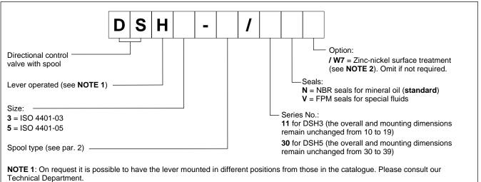
NOTE 2: Standard surface treatment: phosphating. The zinc-nickel finishing makes the valve suitable to ensure a salt spray resistance up to 600 hours.
