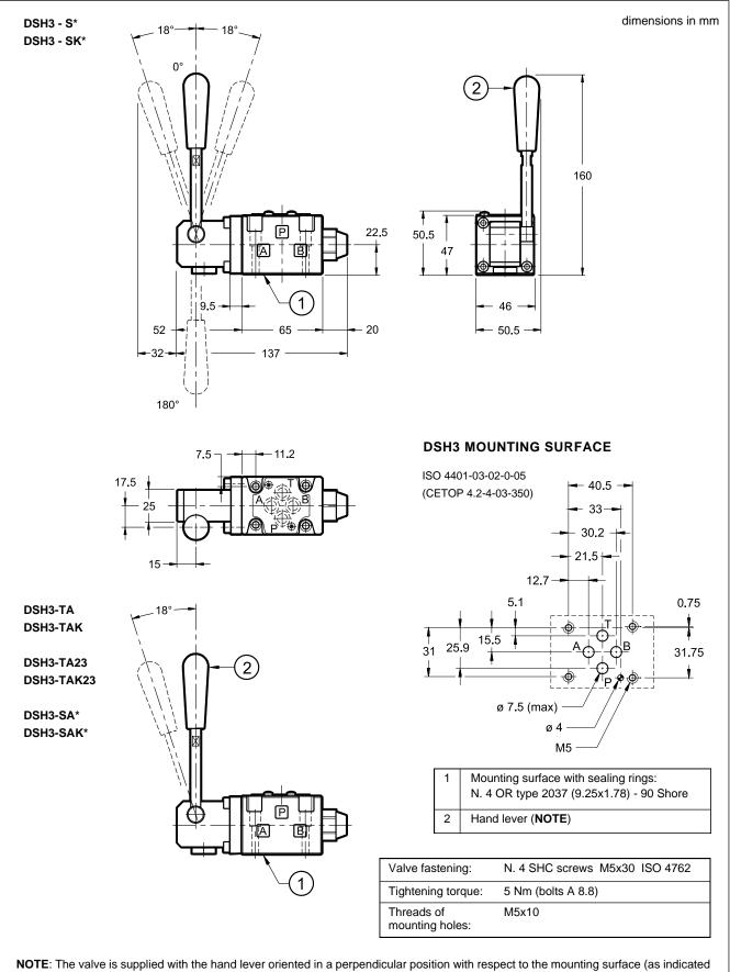
in the above drawing). For installation needs the hand lever can be oriented by the user directly at 180° to the standard position, simply by unscrewing the lever and re-screwing it in the desired position.
