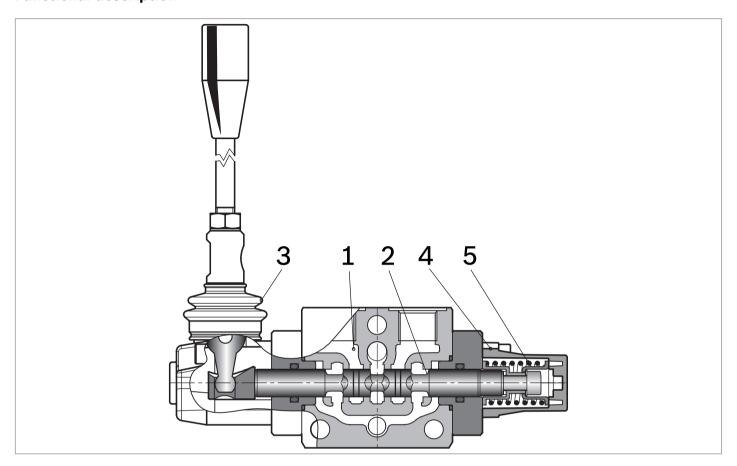
The sandwich plate design directional valve elements L8\_1... are compact manual operated valves which control the start, the stop and the direction of the oil flow.
