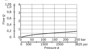
Version: pressure drop  $\Delta p = \Delta p(Q) \ (P_{IN} - P_{OUT})$  to the next section psi bar
