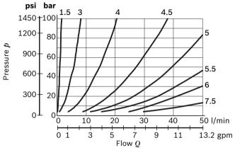
$\Delta p$  curve vs. free flow, through the check valve
