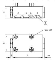
1 Sealing of the ports with O-ring NBR 90 Sh (see table)
