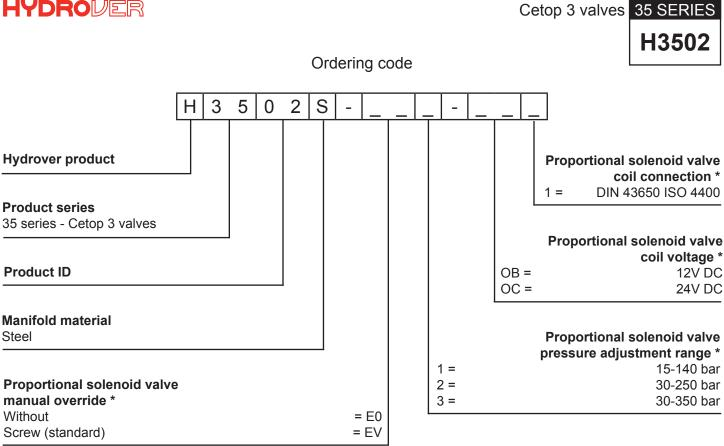
\* Omit if not required. For example, to order the product without the proportional solenoid cartridge valve, omit the manual override, pressure range, coil voltage and coil connection options: H3502S. The manifold will still be provided with the corrisponding cavity.
