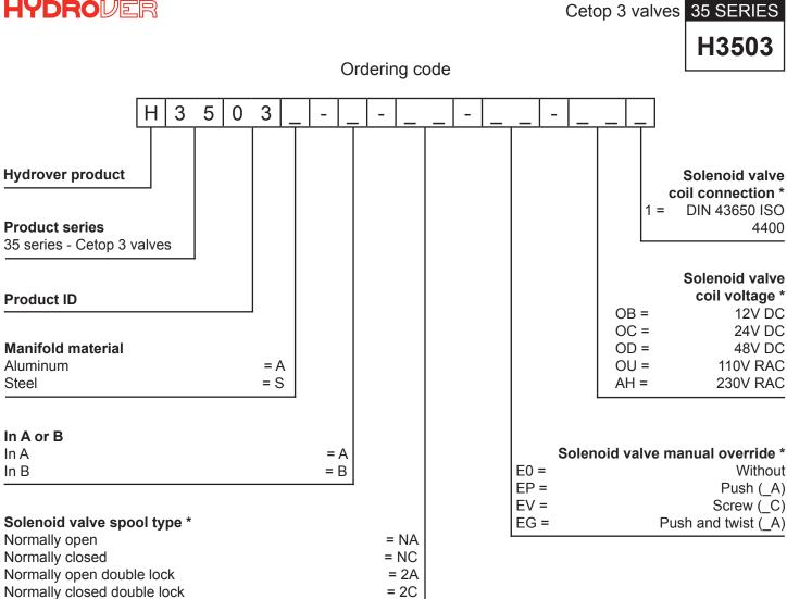
\* Omit if not required. For example, to order the product without the solenoid cartridge valve coil, omit the coil voltage and coil connection options: H3503A-A-NC-E0.
