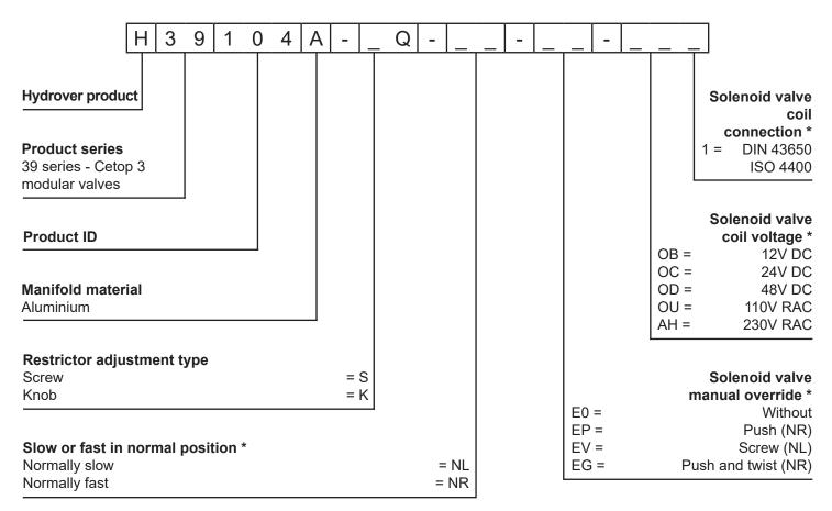
\* Omit if not required. For example, to order the product without the relief cartridge valve, omit the relief valve adjustment type and pressure range options: H39104A-SQ.
