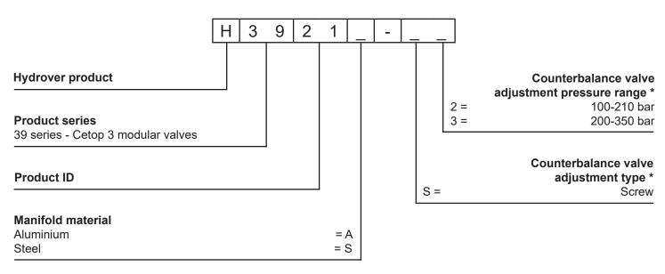
\* Omit if not required. To order the product without the counterbalance cartridge valve, omit the adjustment type and pressure range options: H3921A.
