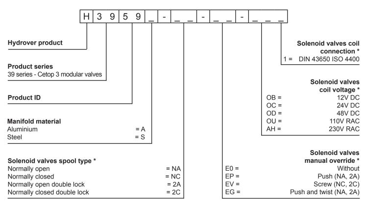
\* Omit if not required. For example, to order the product without coils, omit the solenoid valves coil connection and coil voltage options: H3959A-NC-E0.
