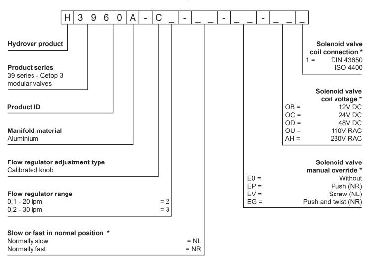
\* Omit if not required. For example, to order the product without the fast slow solenoid cartridge valve, omit the solenoid valve manual override, coil voltage and coil connection options: H3960A-C2.
