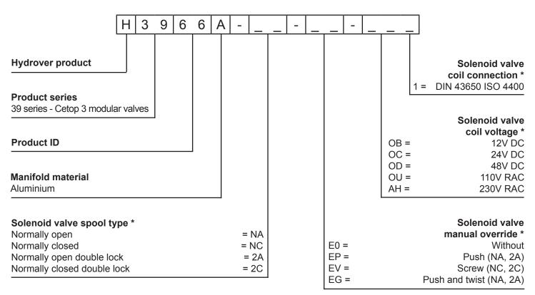
\* Omit if not required. For example, to order the product without coil, omit the solenoid valve coil connection and coil voltage options: H3966A-NC-E0.
