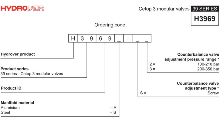
\* Omit if not required. To order the product without the counterbalance cartridge valve, omit the adjustment type and pressure range options: H3969A. The manifold will still be provided with the corrisponding cavity.
