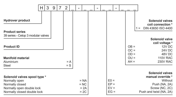
\* Omit if not required. For example, to order the product without coils, omit the solenoid valves coil connection and coil voltage options: H3972A-NC-E0.
