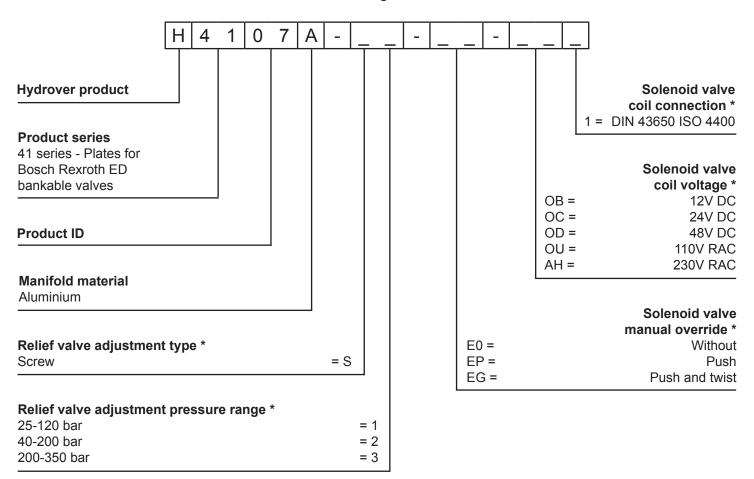
\* Omit if not required. For example, to order the product without the bypass solenoid cartridge valve, omit the coil connection, coil voltage and manual override options: H4107A-S2.
