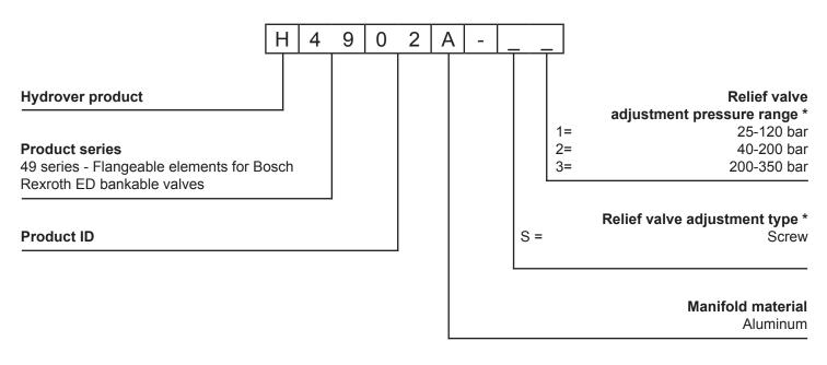
\* Omit if not required. The manifold will still be provided with the corrisponding cavity.
