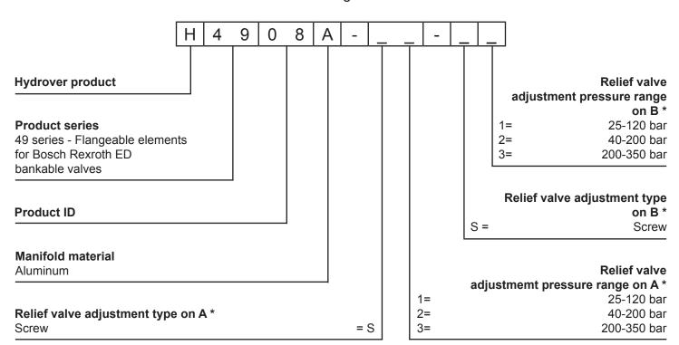
\* Omit if not required. The manifold will still be provided with the corrisponding cavity.
