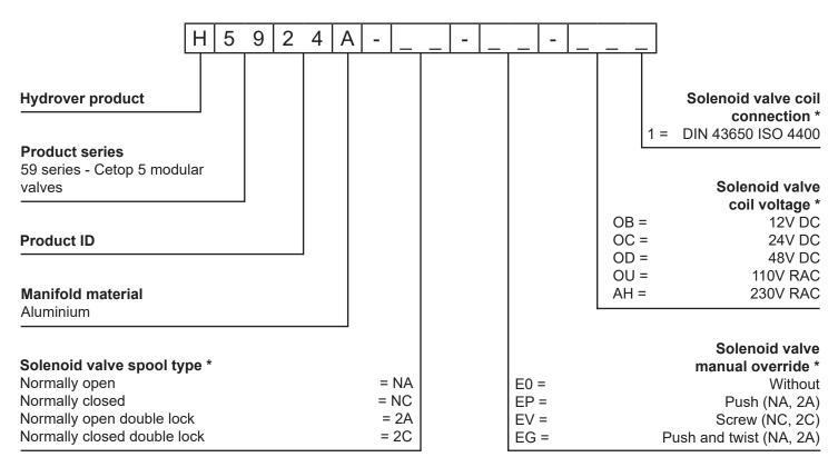
\* Omit if not required. For example, to order the product without coil, omit the solenoid valve coil connection and coil voltage options: H5924A-NC-E0.
