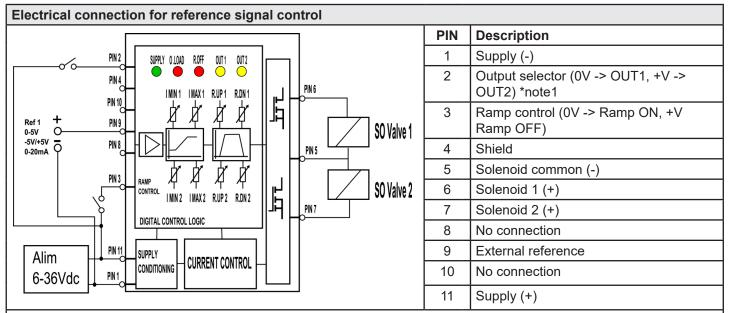
\*Note1: in case of +5V/-5V input control signal, pin 2 works as output enable, in all other case pin 2 works as output selector.
