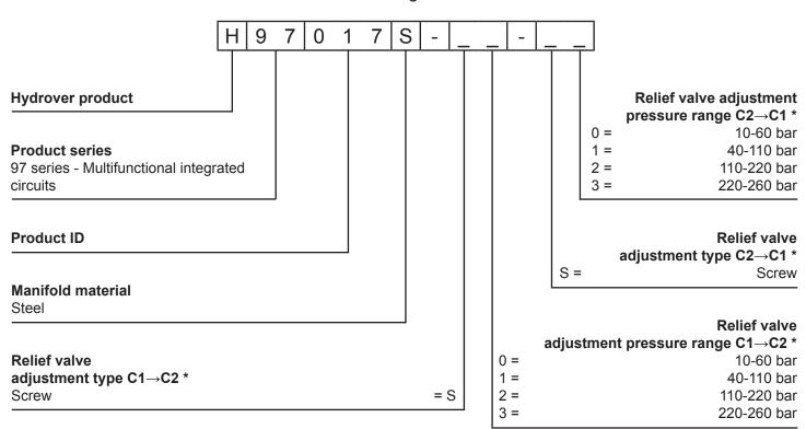
\* Omit if not required. To order the product without the pressure relief cartridge valves, omit the pressure range and the adjustment type options: H97017S. The manifold will still be provided with the corrisponding cavities.
