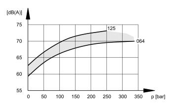
The noise pressure levels were measured in a semi-anechoic room, at an axial distance of 1 m from the pump.
