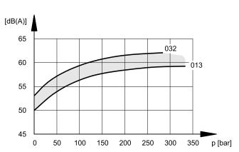
The noise pressure levels were measured in a semi-anechoic room, at an axial distance of 1 m from the pump.
