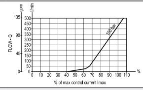
Above 250 bar (3625 psi) deltap the opening point will occur at higher current and flow capacity will be reduced.
