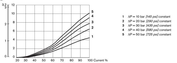
Ordering code S3: it supplies 4 I/min [1.06 gpm] nominal flow at 100% duty cycle, with 10 bar [145 psi] pressure drop. gpm I/min
