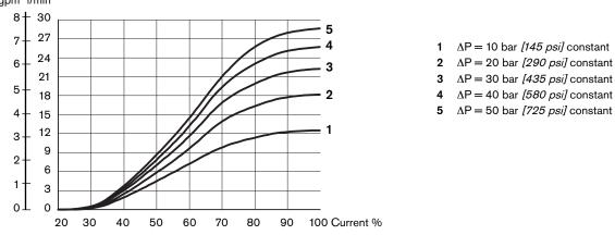
$\Delta P$  = valve pressure differential (inlet pressure minus load pressure and minus return pressure) The characteristic curves are obtained with 4 way connected, P $\rightarrow$ A / B $\rightarrow$ T or P $\rightarrow$ B / A $\rightarrow$ T.
