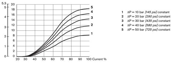
Ordering code S5: it supplies 12 I/min [3.17 gpm] nominal flow at 100% duty cycle, with 10 bar [145 psi] pressure drop. gpm I/min
