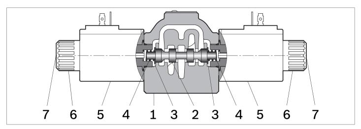
The directional valves LC1F\_DZ are compact direct operated solenoid valves which control the start, the stop, the direction of the oil flow. They basically consist of a housing (1) with a control spool (2), one or two solenoids (5), and one or two return springs (4).
