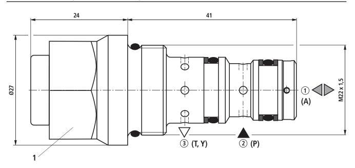
1 Hexagon 24 A/F, tightening torque  $M_T = 60 \pm 5$  Nm
