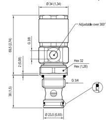
▼ Version 31: Directional control valves pneumatic operated poppet 2-way double lock normally closed - Special cavity
