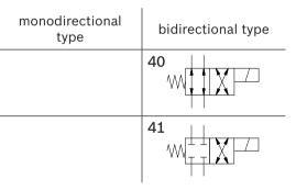
Solenoid operated valves, direct acting spool type 4-way 2-position
