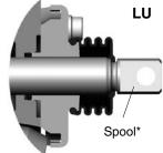
MJA Lever bracket and link parts for mechanical joystick, type A, and for open spool end. Lever bracket MJA have always to be selected in the left section and lever bracket MJ in the right section. Lever itself not included. Must be ordered separately (see page 33).
