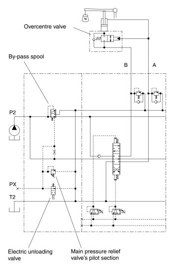
Circuit diagram for pump unloading
