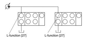
Parallel connection, variable pump (CPU, LS), P70CP, P70LS
