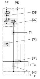
Tank connection T3 open. Free-flow gallery connected with tank via counter pressure function, PT [33].
