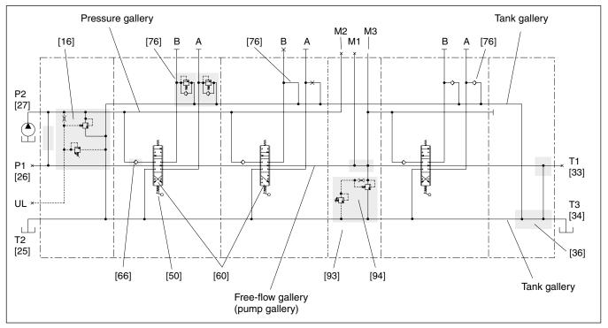
The circuit diagram above shows the P70CF with three spool sections and a mid-inlet between sections 2 and 3.
