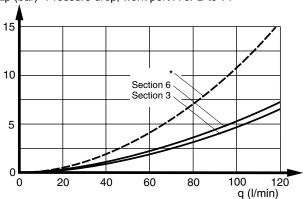
\* Broken line illustrates example of pressure drop in P70CF over a D-spool for q=65 l/min in section 6.
