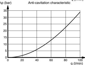
The curve shows the pressure drop between the tank connection and work port when port relief valve (PA) or anti-cavitation valve (N2) without port-relief function is used as an anti-cavitation valve.
