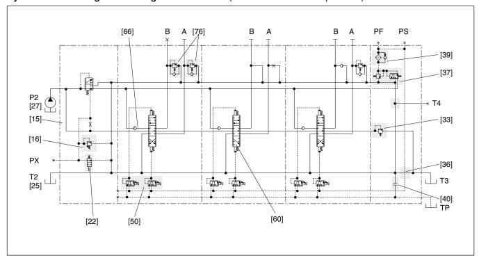
The circuit diagram above shows the P70 with three electrohydraulically controlled spool sections and an integrated pilot-oil supply. The shaded areas indicate functions or function groups that are described further on in the catalogue.
