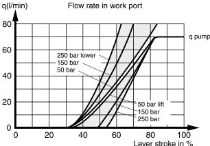
In P70CF valves with hand-operated spools, speed is affected by the weight of the load, i.e. the heavier the lift load, the longer the lever stroke needed before the load starts to move. Conversely, the heavier the load to be lowered, the faster the lowering sequence.
