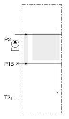
Standard inlet I without main pressure relief valve (P70CF).
