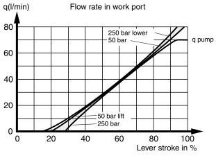
In the P70CF equipped with FPC, PC, ECS and ECH closed spool-actuators, the spools are pressure compensated, with the result that the load's influence on speed is negligible.
