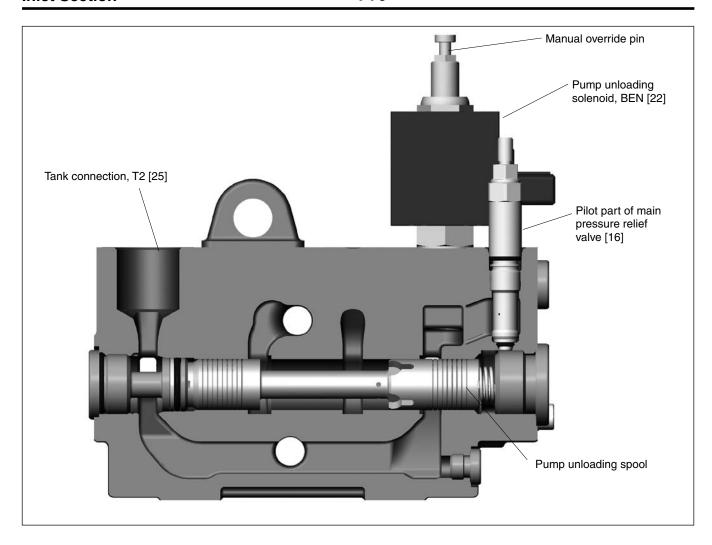
Inlet section for valve with integrated pump unloading function.
