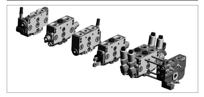
The P70 directional valve is of modular construction. It is designed for many different applications and used extensively in machines such as lorry cranes, miniexcavators, small wheeled loaders and concrete placing cranes. The P70 is available in three different versions: the P70CF with an open centre for fixed pumps, the P70CP with a closed centre for variable displacement pumps and the P70LS with a closed centre, coupled with a load sensing signal, to the variable displacement pump.
