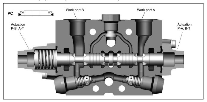
PC Hydraulic, proportionally controlled, spring-centred spool actuator. Best controlled by PCL4 remote control valve (see separate brochure).
