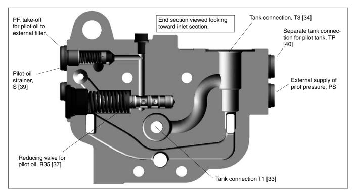
End section with integral pilot-oil supply
