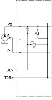
Circuit for inlet section with CUI
