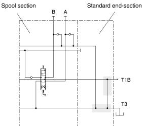
Tank connection T3 open. Free-flow gallery connected with tank gallery in the end section.
