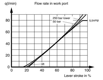
In the P70LS equipped with PC, ECS and ECH closed spoolactuators, the spools are pressure compensated, with the result that the load's influence on speed is negligible.
