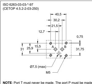
${\bf NOTE}:$  Port T must never be made. The port P must be made only for RPC1 - \*/CTX. Conversion plates are available.
