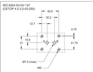
**NOTE**: The RPCED1 mounting interface, with ISO 6263-03 holes, must not have P and T ports or must have the 0113388 subplate (to be ordered separately).
