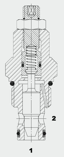
The needle valve SDR10A-11 with reverse flow check is an adjustable, hydraulically operated, spring-loaded spool valve. Depending on the throttle setting, the valve controls the flow rate from port 2 to 1. There is free flow from port 1 to 2. Flow is not pressurecompensated, i.e. the flow rate is dependent on the viscosity and the pressure drop.
