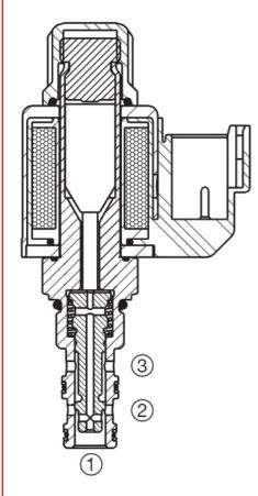
flow from port 1 to 2 and in the opposite direction. Port 3 is closed. If energized, the valve allows flow from port 2 to 3 and in the opposite direction. Port 1 is closed.
