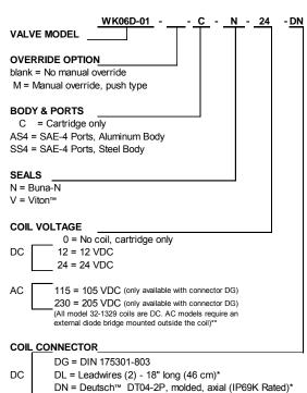
Use mating plug DIN 43650 form B without diode bridge for DC voltages PIN 02600570 Use mating plug DIN 43650 form B w/ diode bridge for AC voltages PIN 02600582 \*\*Mating plugs sold separately
