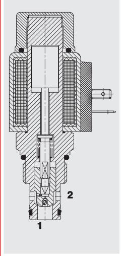
The directional valve is a pilot operated valve in poppet style.
