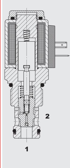
The directional valve is a pilot operated valve in poppet style.
